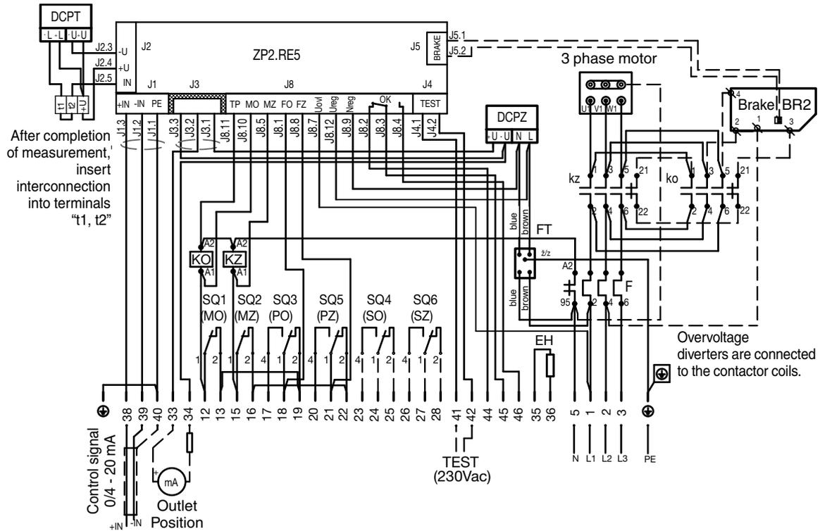
Wiring diagram of electric actuators **MODACT MPS, MPSP Control, T. No. 52 261- 6,**
