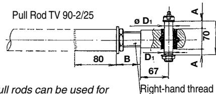
These pull rods can be used for MPR actuators, Type No. 52 223.
