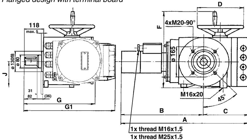
**Note:** Threads for cable bushings in the terminal box: 1 x M25 x 1.5, 3 x M20 x 1.5 (cable bushings are included – attached).
