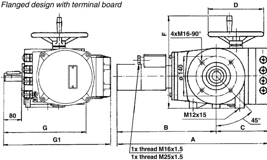
**Note:** Threads for cable bushings in the terminal box: 1 x M25 x 1.5, 3 x M20 x 1.5 (cable bushings are included – attached).
