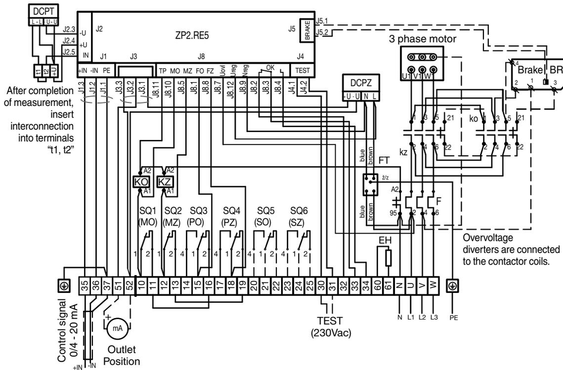
Wiring diagram of electric actuators **MODACT MPS, MPSP Control, T. No. 52 261- 6**
