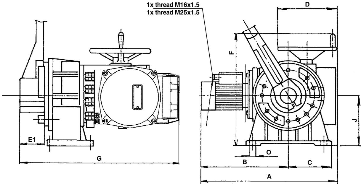
**Note:** Threads for cable bushings in the terminal box: 1 x M25 x 1.5, 3 x M20 x 1.5 (cable bushings are included – attached).
