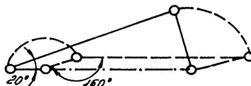
Fig. 7 - *Working stroke of the actuator lever with pull rod*
