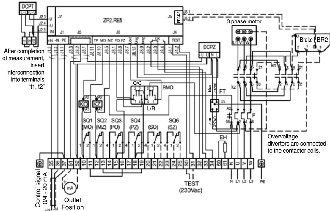
Wiring diagram of electric actuators **MODACT MPS, MPSP**
