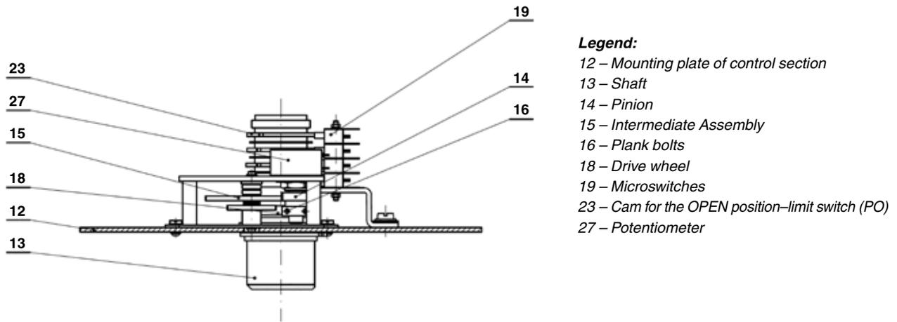
Fig. 6a – **Connection of resistive transmitter with drive in actuators 52 260**
