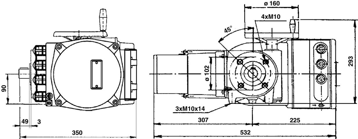
**Note:** Threads for cable bushings in the terminal box: 1 x M25 x 1.5, 3 x M20 x 1.5 (cable bushings are included – attached).
