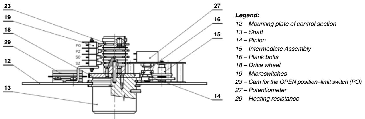
Fig. 6b – **Connection of resistive transmitter with drive in actuators 52 261–52 266**
