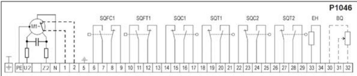
*Design with passive current position transmitter*
