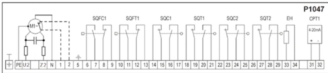
*Design with active current position transmitter (with power source)*
