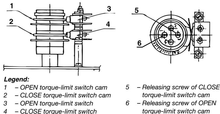
Fig. 3 - Torque-limit switches
