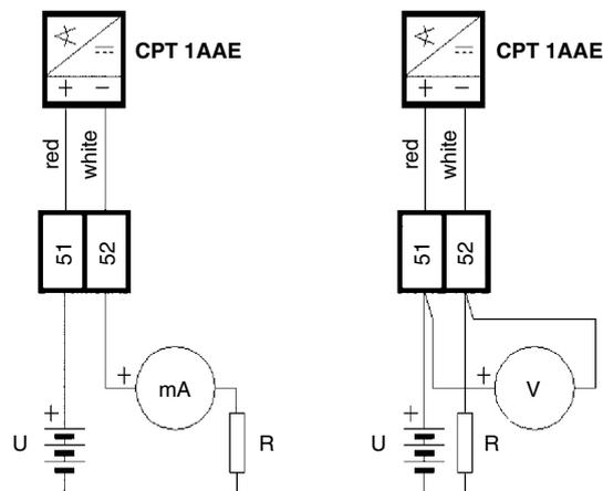
1. Move the output shaft to Closed position. During closing, the current signal value should decrease. If it is increasing, unfix the transmitter body and move to decreasing part of output characteristics by turning of circa 180 degrees. Set 4mA by slight turning. Tighten the shim plates to secure the transmitter against spontaneous turning.
