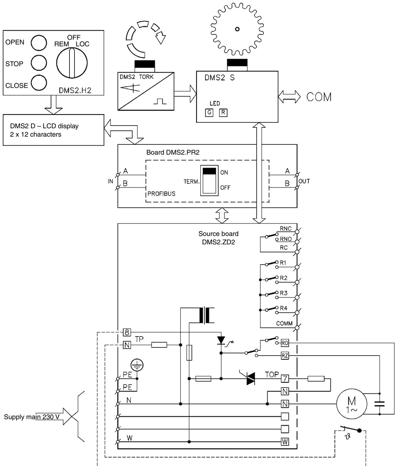
Example of wiring diagram of system **DMS2** in version for control with signals "open" and "close" or in version for control with analog current signal with three-phase electric motor
