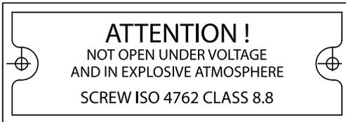
4) Plates on covers with marking of used protection against explosion
