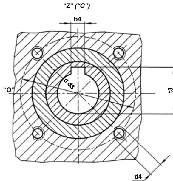
The position of groove for keyway according to ISO 5211 and DIN 3337 is in the position "Closed". The position "Opened" is to the left of the position "Closed" when viewing in the direction to the local indicator of position. The position "Z" ("C") of the groove for keyway is identical with the position "Z" ("C") on the local indicator of position.
