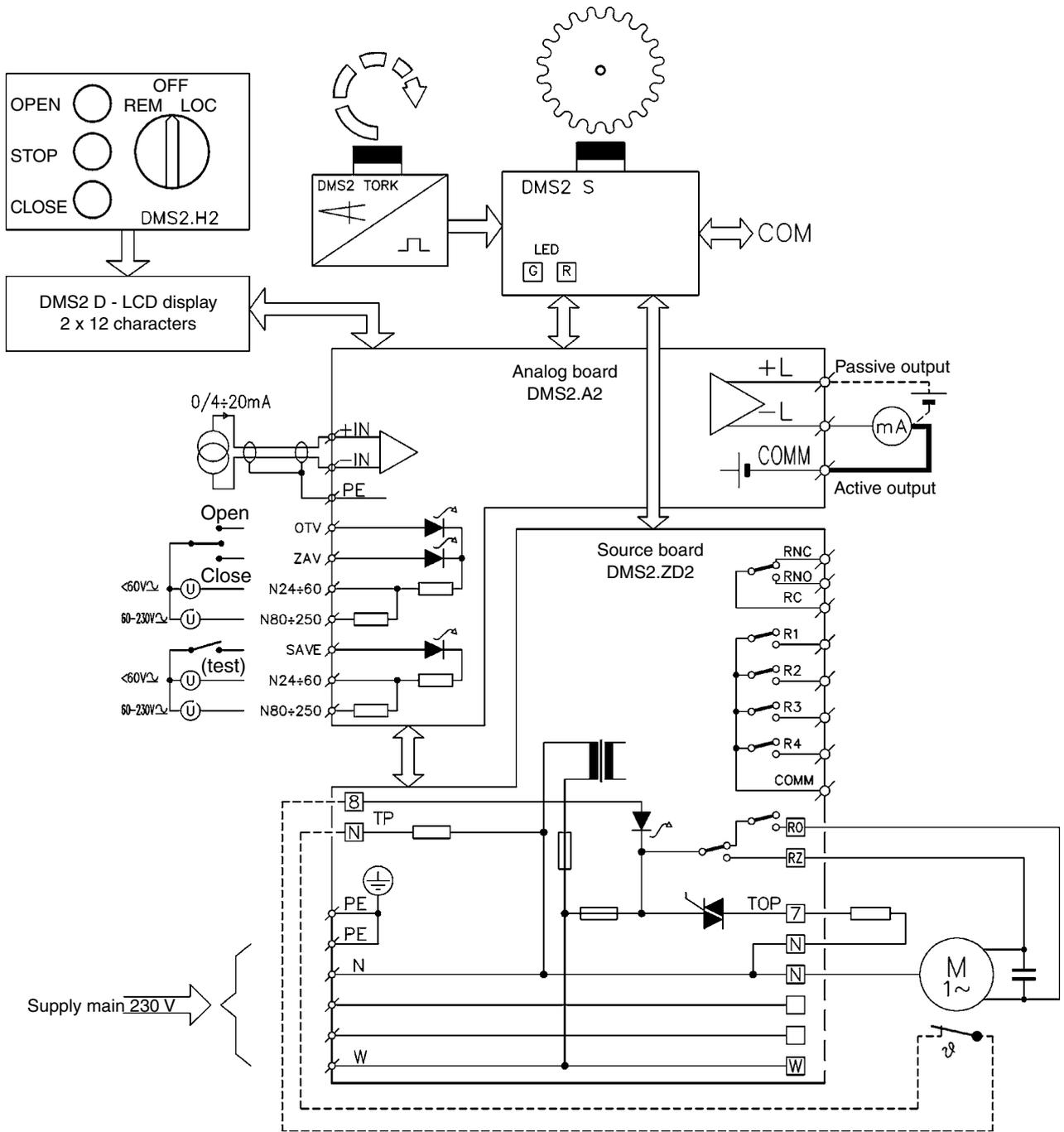
Example of wiring diagram of system **DMS2** in version Profibus with single-phase electric motor
