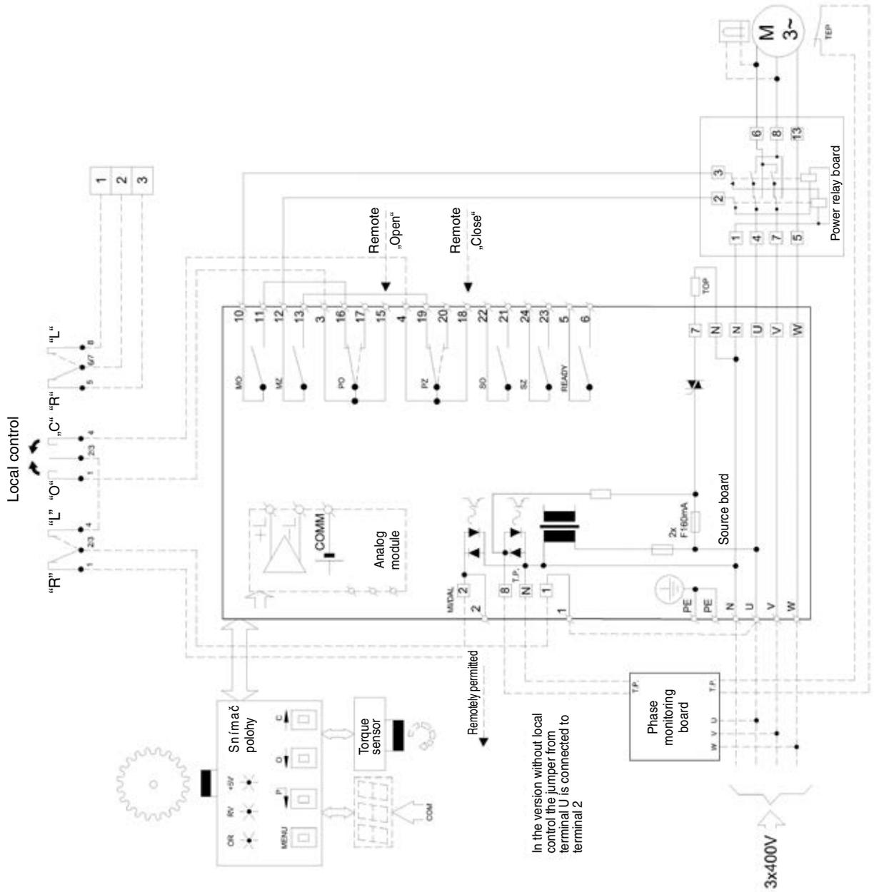
Example of wiring diagram of electronics **DMS2 ED** in version **Control** with single-phase electric motor
