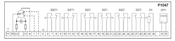
Design with active current position transmitter (with power source)
